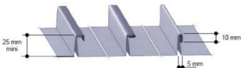
Figure 19 – Pliage du joint debout
