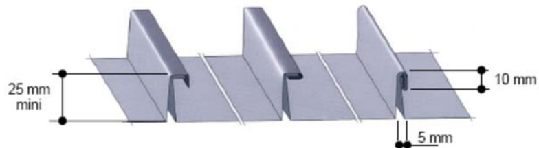
Figure 4 – Pliage du joint debout
